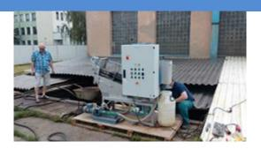
Volute ES-131 managed to dewater all types of imported sludge from a Czech company collecting and treating this sludge from various car and truck wash facilities. With a proper polymer and the right dosage Volute reached very satisfying results in dryness and clean filtrate as well for the customer. The clog-free construction is a perfect feature for this oily and greasy sludge.
